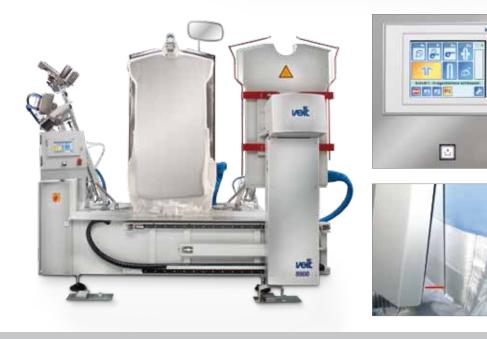
The VEIT-Touch-Control is equipped with a 5.7" touch-screen colour display which shows all functions and parameters at one glance. Steam and dry times as well as the programs can be changed easily. Service and maintenance functions can be controlled manually with the touch-screen display.
