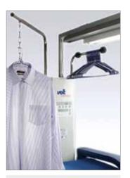
The swivel tube with chain for quality control and touch up as well as the ergonomically fixed hanger suspension are important details of an universal ironing table.
