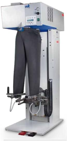
VEIT PANTS FINISHER 8741 LONGITUDINAL TENSIONER The basic version of the Pants Finisher with longitudinal tensioner provides a rational and low-cost finishing of short and long trousers. The standard equipped inner and outer tensioner, the anti-stretch in the longitudinal tensioning as well as a strong warm-air-fan guarantee an excellent price-performance ratio.
