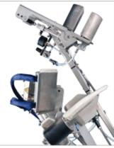
The sleeve tensioners for short and long sleeves come with pneumatic height adjustment. The heat accumulation plate ensures fast drying of the seams. With the new optional cuff-tuck-press sleeves get perfectly finished.
