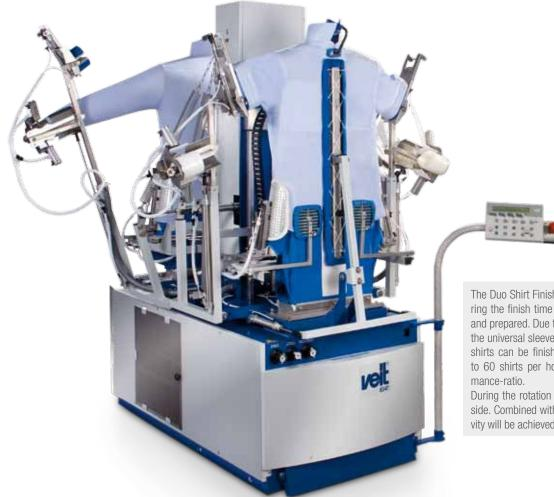
The Duo Shirt Finisher consists of two rotating bodies. During the finish time of one shirt the other shirt is clamped and prepared. Due to the established blowing principle and the universal sleeve tensioning device, short or long sleeve shirts can be finished mixed. The high productivity of up to 60 shirts per hour provides an excellent price-performance-ratio.
