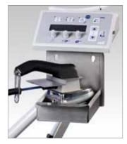
The automatic side vent fixing device is not only used on side vents, but is used generally for fixing the shirt or smock seams.
