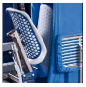
The ham clamp unit, especially pervious to air for fast drying of the side seams and crease-free fixation of the shirt hem.
