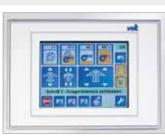
The VEIT-Touch-Control is equipped with a 5.7" touch-screen colour display which shows all functions and parameters at one glance. Service and maintenance functions can be controlled manually with the touch-screen display.
