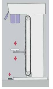
THE PATENTED DRIVE SYSTEM combined with the integrated Anti-Stretch-Control provides exact longitudinal tensioning. The VEIT Belt-Drive-System provides a smooth and gentle movement of the hem clamp unit. The clamping position, from long pants to shorts, can be changed automatically by using the foot switch. The manual adjustment of the carriage from long pants to shorts is no longer necessary.
