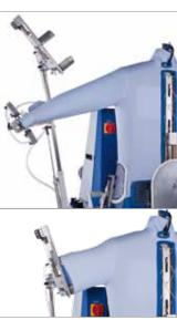
Long sleeve and short sleeve shirts can be fixed without marks with the drop shaped sleeve tensioner. The pneumatic height adjustment of the sleeve tensioner can be controlled on the control panel for one side or both sides together.
