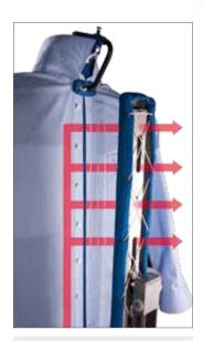
Fast and energy-efficient drying of the button-facing with VEIT-Direct-Airflow, through the separate air flow in combination with the powerful fan and heating register.
