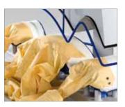
The built in vacuum in the lower bucks guarantee a safe positioning of the cuffs and collar.
