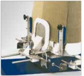
SIDE VENT CLAMP FIXING APPLIANCE VEIT 8362 Side vent clamp fixing for jackets allows an easy finish without marks on jackets.
