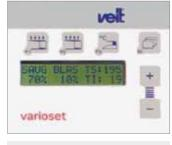
Quick regulation of suction and blowing quantity by key pressure on the electronic control unit. Rated and actual temperature of the iron is shown accurately to the degree.
