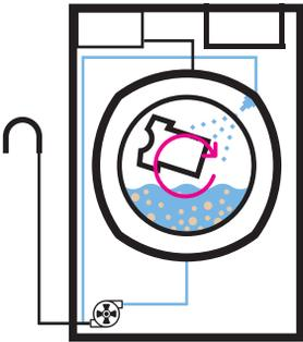
The water-detergent mixture is pumped from the bottom of the caustic tank and sprayed specifically onto the laundry. This makes the detergent dissolve better and ensures an optimal washing effect.
