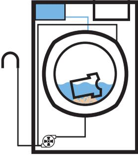
The washing programme starts: The detergent compartment is rinsed with water and the drum flooded.
