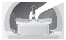
Pull the fluff filter out of the filter support.
