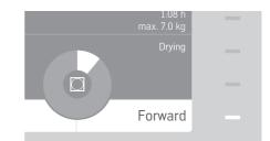
Press the light bar next to Forward until the desired programme step is displayed.
