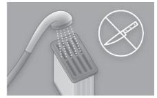
Rinse the slots of the air cooler from the front side with running water.
